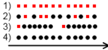
Figure 4.1: An overview of different execution trace organisations. 1) All significant events, 2) Evenly spread events, 3) Clustered events and 4) No significant events. Normal events are black circles. Significant events are red squares.
